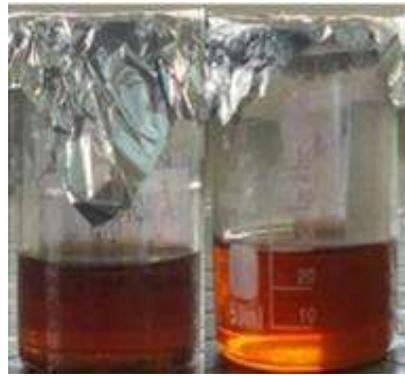
**Figure 2.5:** a) Engine oil+ graphite nanoplatelets (GrNP), b) Engine oil (without graphene nanoplatelets (GrNP)- (Day 7)
