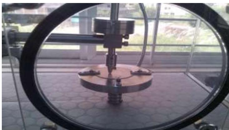
**Figure 1.3:** Diagram showing substrate holder and pin (IST)
