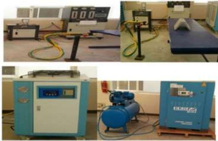
**Figure 1.1:** HVOF Sulzer Metco with water cooled diamond jet gun DJ8A hardware 2600 (IST)
