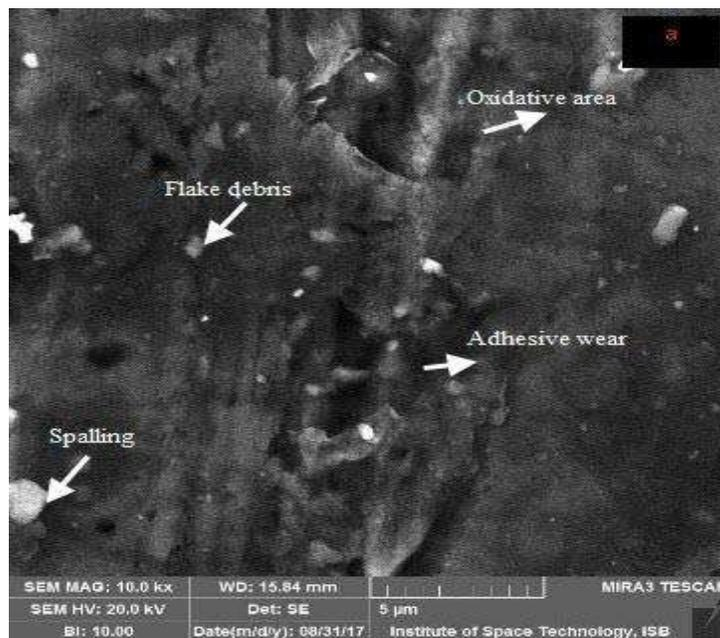
**Figure 2.9:** SEM image of graphite nanoplatelets (GrNP)+ engine oil dispersed on WC-10Co-4Cr coating
