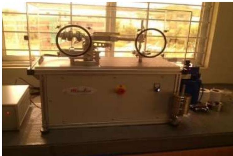
**Figure 1.2:** Pin-on-disk tribometer 10.2 (IST)
